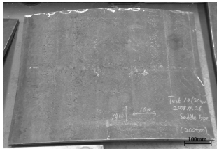
Fig. 9. Forming test for a saddle type plate using a flexible forming apparatus.
