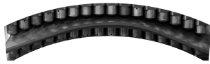
Fig. 8. Forming test for a saddle type plate using a flexible forming apparatus.
